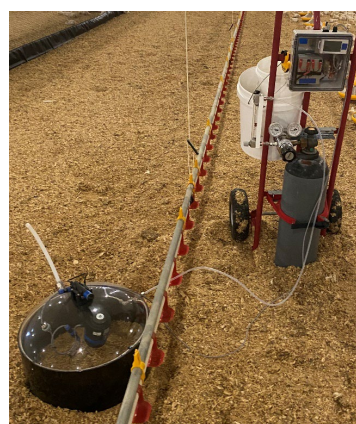
Figure 2 - Isolation chamber with ammonia ( \text{NH}_3 ) sensor to measure emissions from the litter.
