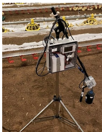
Figure 1 - In-shed sensor stand with data logger and sensors to measure ammonia ( \text{NH}_3 ), temperature and relative humidity.
